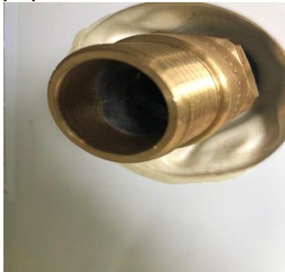
**Sealing compound product must be let set for 4 hours before allowing water pressure to build up in machine.**
